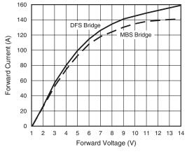
Figure 1. Forward Current vs. Forward Voltage
