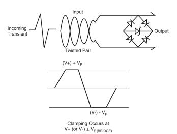
Figure 6. shows an alternate method of using a SMD bridge to provide effective low loss protection for "twisted pair" arrangements.
